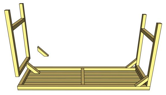
Once each bracket is secure, turn the unit upright and position the bottom shelf like so:
